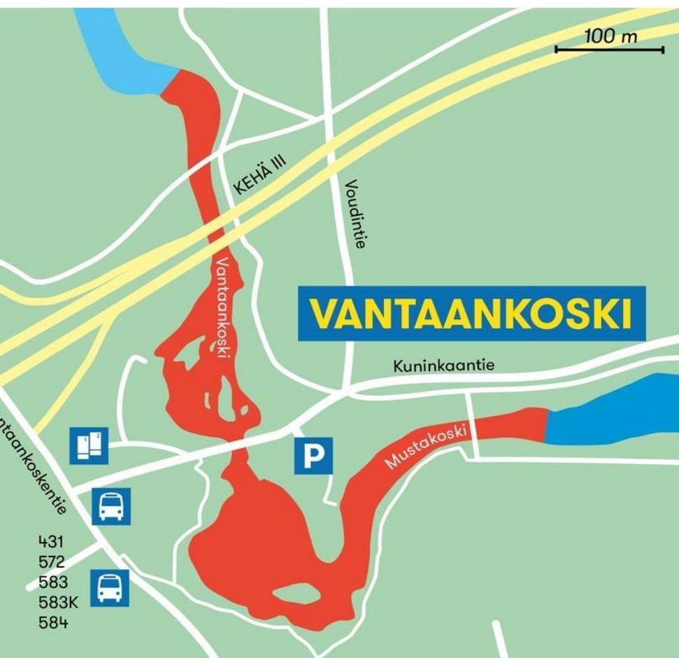
**Vantaankoski** is 400 meters long with a drop height of 5 meters. The average flow is around 12 m<sup>3</sup>/s, but the flow varies to a significant extent. Mustakoski is 250 meters long with a drop height of around 1 meter.
