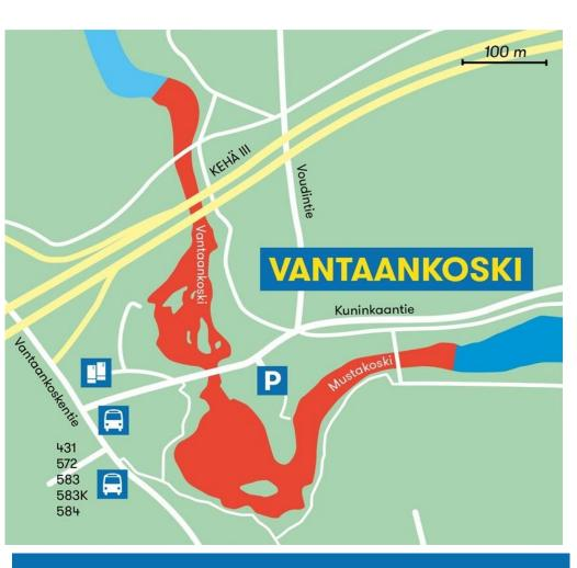
**Vantaankoski** is 400 meters long with a drop height of 5 meters. The average flow is around 12 m3/s, but the flow varies to a significant extent. Mustakoski is 250 meters long with a drop height of around 1 meter.
